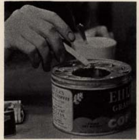
Above: The only kind of an ash tray crewmen aboard many tugs believe is worth having around; a coffee can cut and punched like this. Keeps ashes from blowing out.
