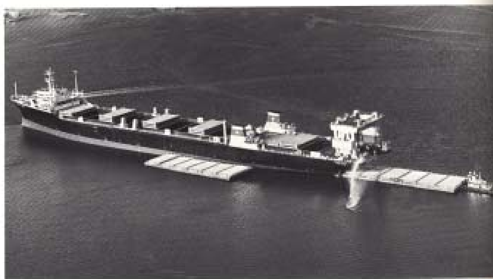
M.V. ACADIA FOREST, the world's first LASH vessel, is a 20-knot, 860-foot-long vessel operated by the Central Gulf Steamship Corporation under a long term time charter for her Norwegian owners. Here she is shown loading barges at Panama City, Florida with her giant 510-ton shipboard gantry crane. Voyages are scheduled between U. S. Gulf ports, the United Kingdom and Western Europe.
