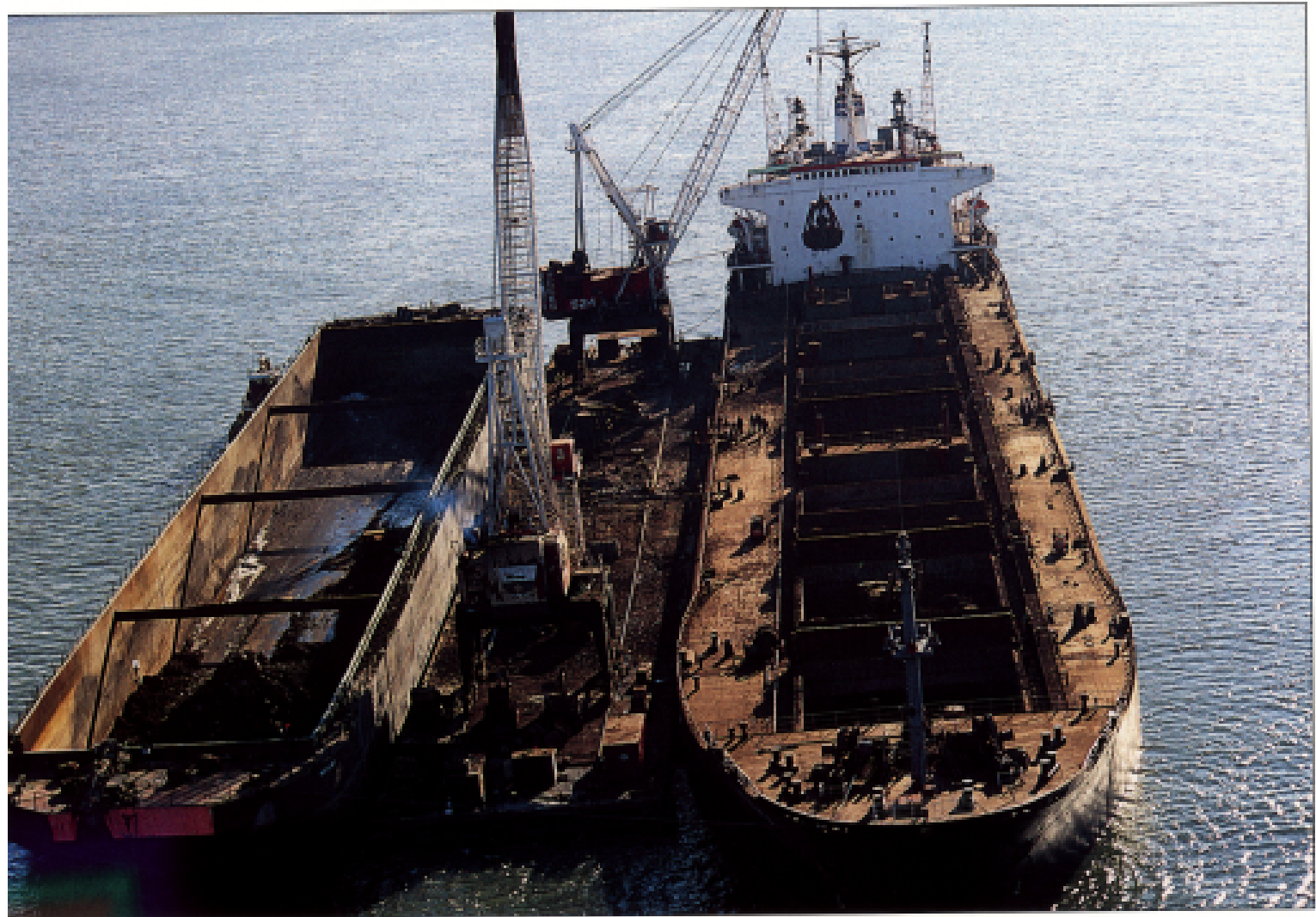
The bulk barge MARYLAND tops off a scrap bulk ship at the Staten Island anchorage in New York Harbor. MARYLAND, with a cargo capacity of 22,800 tons, replaced the former use of ten smaller barges for the same operation.
