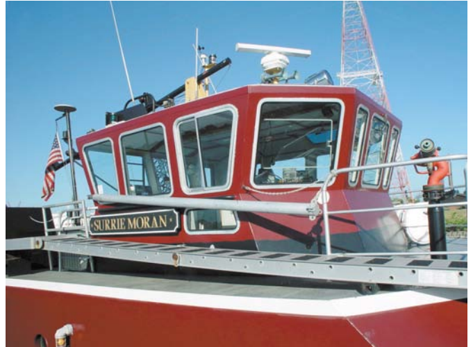
Surrie Moran , a 4,200 hp z-drive tractor tug, is now top tug for MORAN's fleet on Delaware Bay.
