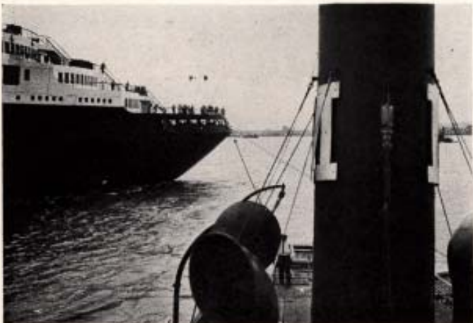
A "team of tugs" pull the stern up stream while others push the bow into the berth.
