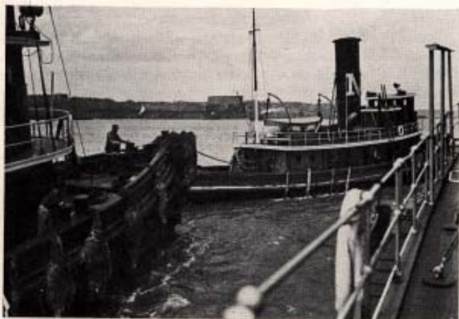
The second tug "anchors" the first. Keeps it from "slipping off" and losing its effectiveness.
