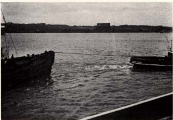
Tugs are hooked together in tandem. Pulling power, if needed, now equals the power of both tugs.
