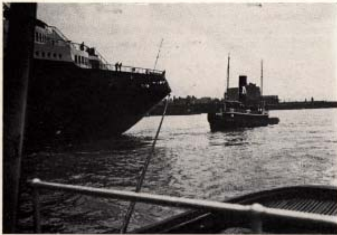
A tug has a line on the stern of the liner. Midway between the tug and the liner a heaving line may be seen in midair.
