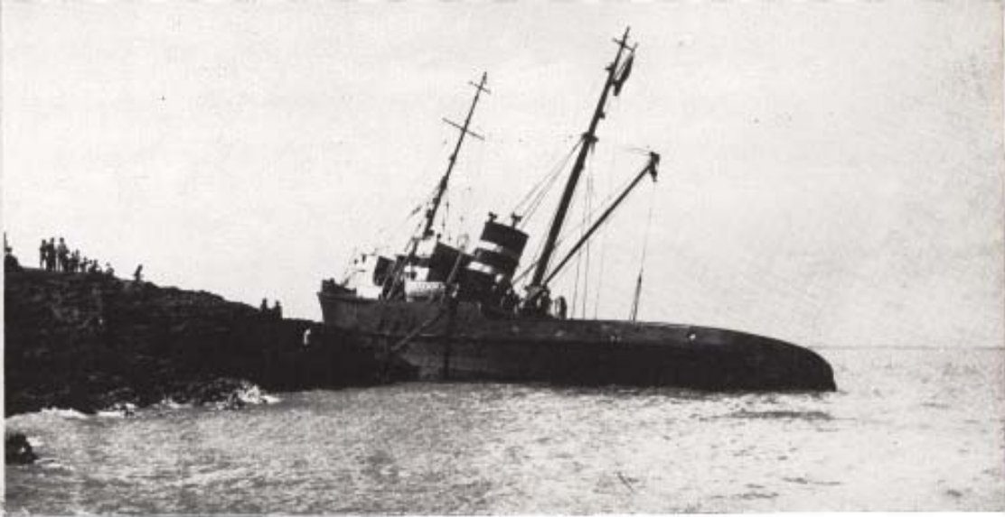
3 . . . The 210-foot, 3000-horsepower Foundation Josephine, apparently hopelessly aground, was about to be abandoned as a total loss. After a salvage crew had patched her bottom, the tug Kevin Moran succeeded in freeing her.
