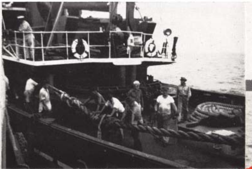
5 . . . With the Canadian tug's huge cable-laid hawser made fast to her bitts, the Kevin prepares to exert the full power of her Diesel-electric engines. Fortunately, good weather prevailed during this critical stage of operations.
