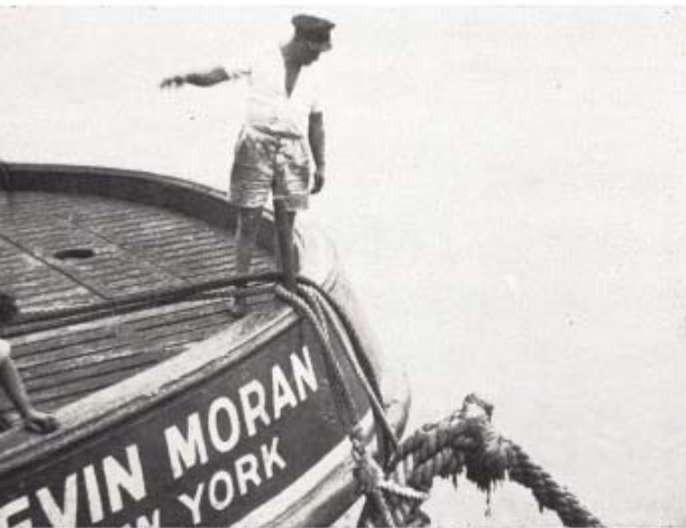
4 . . . The sturdy 143-foot, 1900-horsepower "M" tug, hastily detached from duty in the Gulf of Mexico, is shown here taking aboard the Foundation Josephine's 18-inch hawser after breaking her own pulling on the Leicester.
