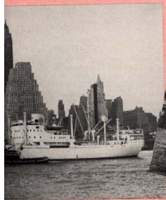
S/S BLIDUM. Nordfriesische Reederei, G.M.B.H., owners. J. Werner, captain. Length, 329 feet; gross tonnage, 1,689; horsepower, 1,200 (turbine); passengers, 8; cargo capacity, 3,403 tons. Service: between North Atlantic U. S. and Gulf-Caribbean ports.
