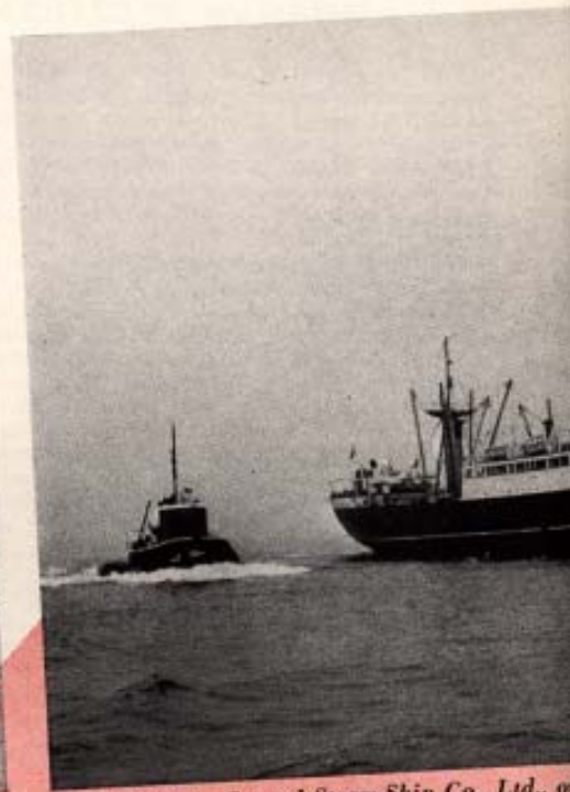
S/S ASIA. Cunard Steam-Ship Co., Ltd., agents. Length, 487 feet; gross tonnage, 8,750; horsepower, 6,500 (turbine). Service: London-Liverpool and Port Alfred-Montreal.
