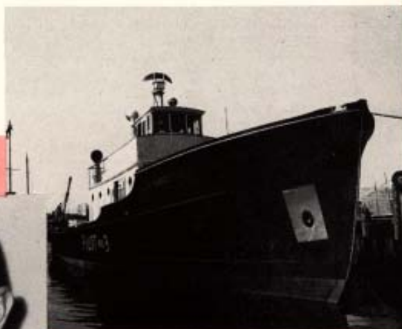
New pilot boat, Sandy Hook: Length, 90 feet; depth, 10 feet (amidship); draft, 7 feet, 10 inches; beam, 18 feet, 11 inches; power, 400-horsepower Caterpillar diesel; crew, 8 men.
