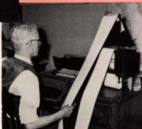
Walter Boylan, senior dispatcher, recording ship movement messages received from New York Custom House by telautograph.
