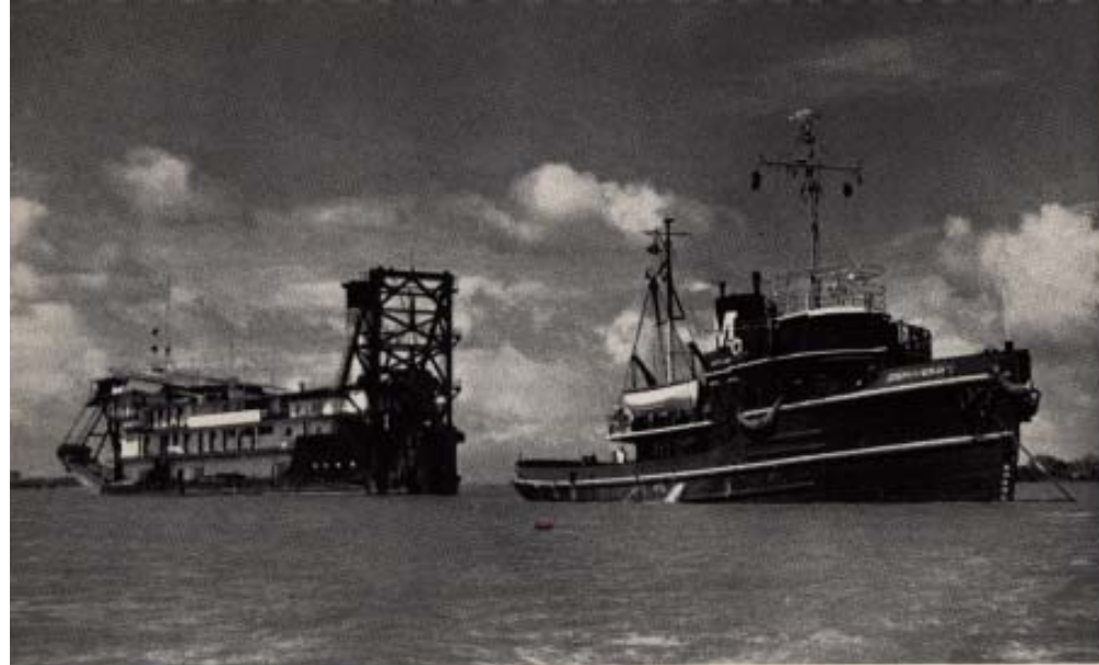
Moran Towing & Transportation Co.'s 1,900-horsepower, diesel-electric ocean tug JOSEPH H. MORAN, II, on her arrival at Puerto Ordaz, Ven., with the CARIBBEAN.
