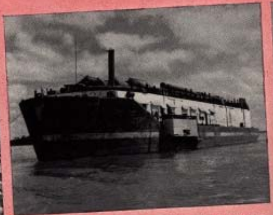
A YF barge fitted up as a machine shop and adequate living quarters was part of the flotilla.
