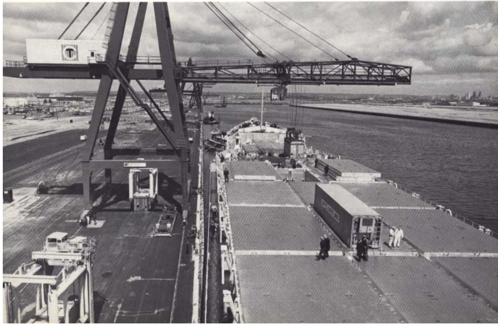
NEW CONTAINER SHIP — The United States Lines' sleek new American Lancer , on her first visit to New York. The 700-foot, 6 inches, vessel has a displacement of 32,000 tons and can carry 1,200 containers. She exceeded 25 knots on her sea trials. With her five sisterships she will serve on the Rotterdam, Hamburg and London range. Note the 4,300-hp. Teresa Moran at the bow of the American Lancer in the picture below.
