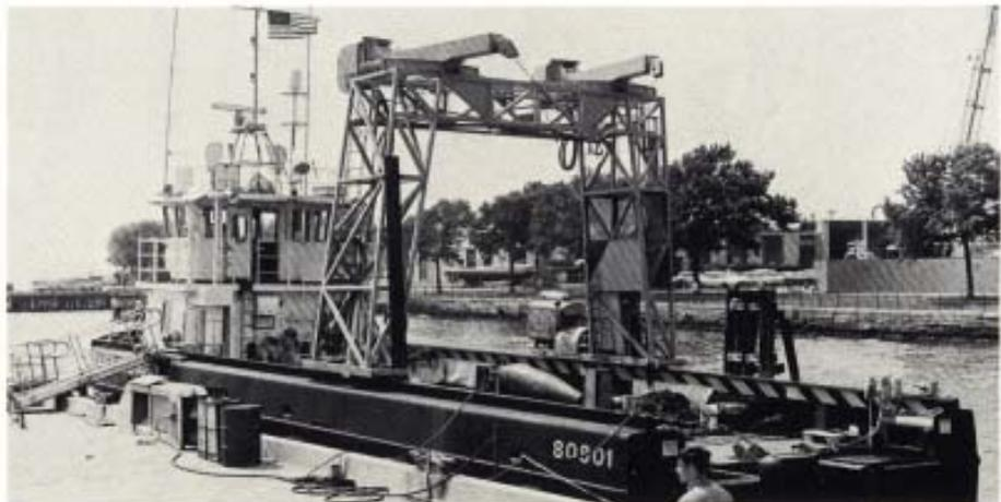
**BUOY TENDER TERN** (WLI-80801), a completely new type buoy tender with an "A" frame for lifting buoys. Master Chief Boatswain Mate T. Crosby is the Officer in Charge.
