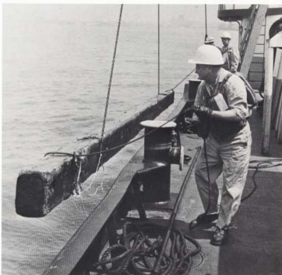
MASSIVE TIMBER —Hoisting a huge piece of wood aboard the Driftmaster is an every-day occurrence. Many propellers have been damaged by hitting such a hazardous piece of floating debris. To the right Driftmaster crewmen bring the timber in from the craft's bow.
