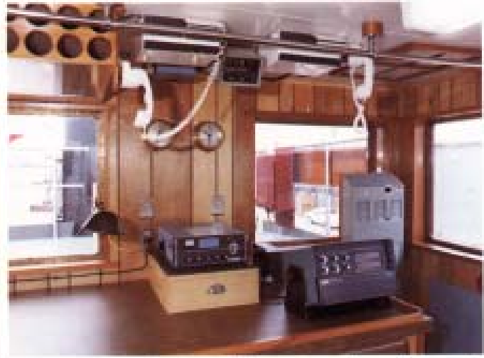
MIRIAM MORAN's wheelhouse control console with dual lever-type steering replacing tug's traditional wheel (Photo, left) and, directly aft, the spacious chart table and communication and navigation electronic equipment (Photo, right).
