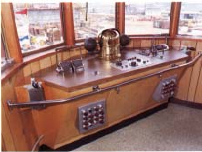
MIRIAM MORAN's wheelhouse control console with dual lever-type steering replacing tug's traditional wheel (Photo, left) and, directly aft, the spacious chart table and communication and navigation electronic equipment (Photo, right).
