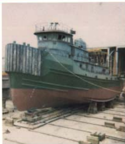
NEW BOW LOOK — The new Doris Moran , shown here on McDermott ways, displays well the individual components of the vertically-hung bow fender system.
