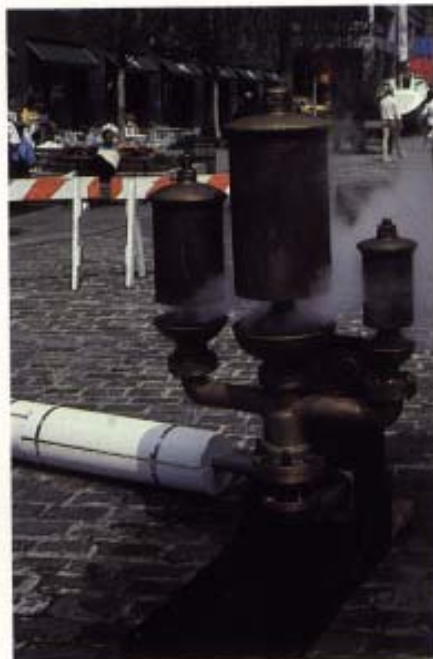
The NORMANDIE'S steam whistle blasts out a 130-decibels, using steam from Con-Edison's underground main at the South Street Seaport Complex.
