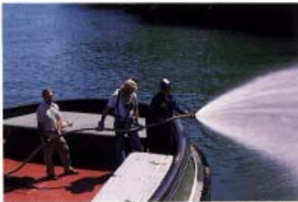
Fire drills include the use of the fire hoses actually putting water over the side. Each tug also has a diesel driven portable pump aboard for emergency use in case the main fire pump is inoperative.
