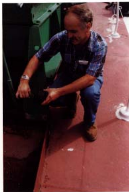
Tom Pearce, port captain for the Moran Services Corp., checks a plug on a tank barges spill rail. All the Moran tank barges have spill rails to catch any deck spills before it can enter the water. On board audits by the port captain and crew of equipment is a major part of the pollution control program.
