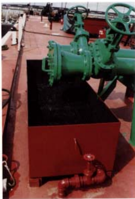
All Moran tank barges are fitted with spill rails and manifold containment boxes to catch any spills.
